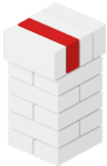
Brick post 25x25 cm coping made of solid brick placed vertically
