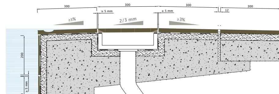
The invisible grid is a new solution patented by Mirage® for recycling water at the poolside. This grid has slots at the side for the passage of water, which are not visible once installed.
